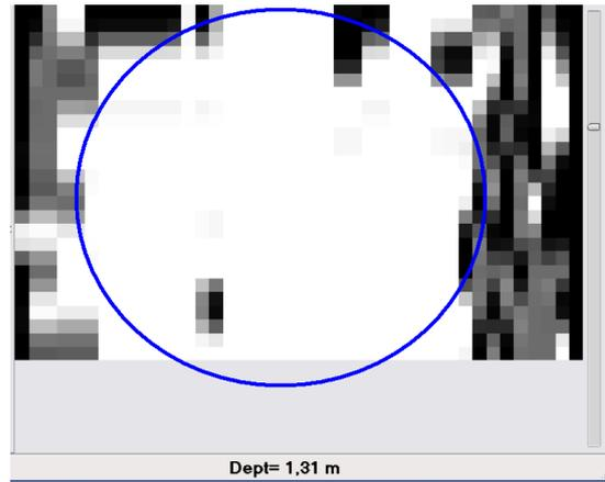
Fig. 4. View from above. Horizontal section of ground, built with 10 parallel profiles. Depth of 1.3 m, corresponding to the depth of standing water surface in the well
